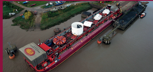
Offloading a tunnel boring machine, consisting of 5 individual loads at Combswich Wharf
